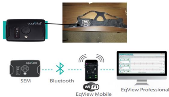
Fig. S2.4. Top: Left Sensor Electronics Module (SEM) inserts into the pocket on the harness. Bottom: from Left to Right: The SEM communicates via Bluetooth to an Android phone with Eqview Mobile installed, which then can communicate to a computer with EqView Professional installed. (Photo and graphic used with permission from the manufacturer).
