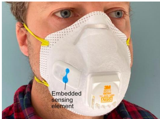
Fig. S5.4. Personal protective equipment with embedded sensing capabilities. These approaches can, for example, include sweat sensors integrated into facemasks that might support an early detection of fever for healthcare workers in contact with potential COVID-19 patients. Courtesy of Epicore Biosystems, Inc., MA, USA.
