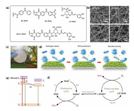
**Figure 9.5** (a) The structure of the daylight active molecules. (b) The morphology of the fibers loaded with the active molecules. (c) Image of the nanofiber samples. (d) Scheme demonstrating the mechanism of action for the antibacterial activity. (e) Diagram demonstrating the excitation of the molecules. (f) The plausible mechanism of the photoactivation. Reproduced with permission from Ref. [55]. Copyright 2018 American Association for the Advancement of Science (CC BY-NC) license.
