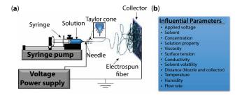
**Figure 9.2** (a) The basic setup for electrospinning technology and (b) the influential parameters on the generated electrospun materials.
