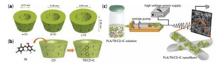
**Figure 9.6** (a) The structures and dimensions of the various cyclodextrin (CD) types. (b) The scheme for the production of the triclosan(Tr)–CD–inclusion complex (IC). (c) The illustration of the strategy for the fabrication of the polylactic acid (PLA)based Tr–CD–IC electrospun nanofibers. Reproduced with permission from Ref. [80]. Copyright 2013 American Chemical Society.
