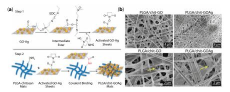
**Figure 9.7** (a) The chemical process for the modification generating GO–Ag functionalized PLGA–chitosan electrospun and (b) the scanning electron microscopy (SEM) images [82]. Copyright 2015 American Chemical Society.
