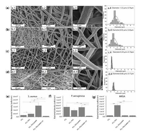
**Figure 9.4** Electrospun nanofibers composed of (a) polycaprolactone (PCL), (b) PCL:polyethylene glycol (PEG), (c) PCL:PEG:gelatin methacryloyl (GelMA), (d) crosslinked PCL:PEG:GelMA. The antibacterial study of the nanofibers for 24 h against (e) *Staphylococcus aureus* (*S. aureus*), (f) *Pseudomonas aeruginosa* (*P. aeruginosa*), (g) *Methicillin resistant Staphylococcus aureus* (MRSA). Reproduced with permission from Ref. [53]. Copyright 2018, De Paula (CC BY) license.
